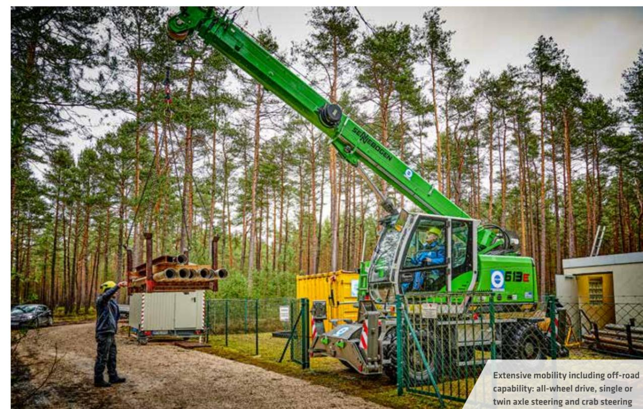
Extensive mobility including off-road capability: all-wheel drive, single or twin axle steering and crab steering
