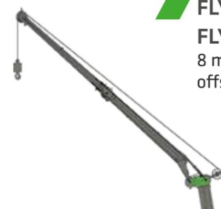
**FLY JIB 8 m, FLY JIB EXTENSION TO 15 m**
