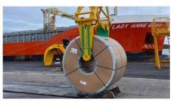
Spreader for steel coils
