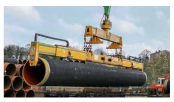
Quick change system with lifting beam
